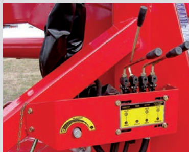
Hydraulic control panel for easy operation for all functions.
