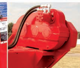
Roll transmission achieved through a sturdy reduction gearbox and only one chain.
