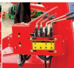
Independent Hydraulic Controls. Speed Control Valve.
