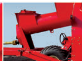
20" diameter auger for big loading capacity.
