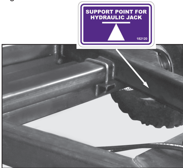
Figure 2 - Support point for jack location
