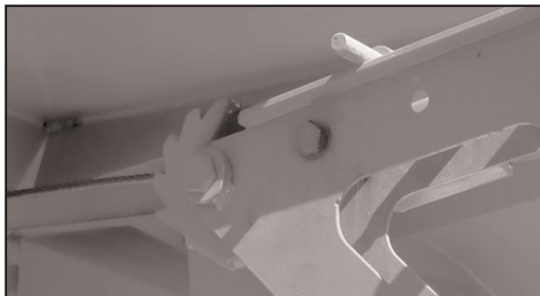
Figure 11 – Cradle fastened by locking lever.
